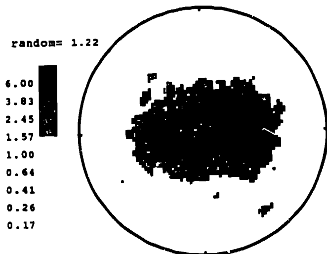
Figure 1. Basal Texture of 1.4 mm thick cross-rolled ingot sheet.
